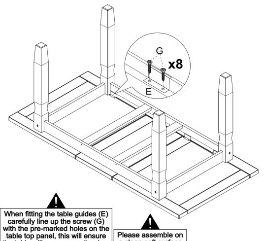
When fitting the table guides (E) carefully line up the screw (G) with the pre-marked holes on the table top panel, this will ensure the table will open correctly when the table requires extending.
