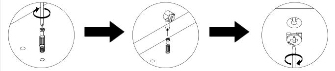
STEP 1 - USE A CROSS SLOT SCREWDRIVER TO TIGHTEN THE CAM BOLT INTO THE HOLE.
