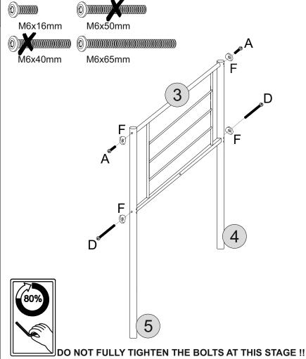
DO NOT FULLY TIGHTEN THE BOLTS AT THIS STAGE!!
