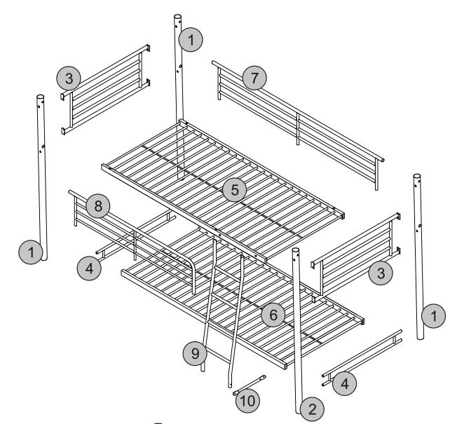
PLEASE NOTE: UPPER BASE 5 HAS HOLES FOR ASSEMBLY OF LADDER AND SAFETY RAILS
