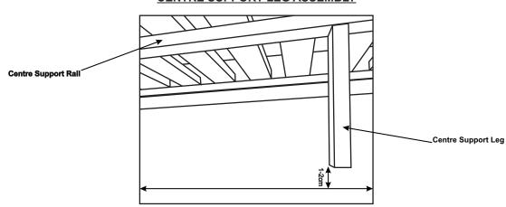
The <u>1-2 cm</u> gap above prevents the centre legs from bending or breaking when weight is quickly redistributed. A shorter interior leg will allow the load of the user to be distributed over the entire load-bearing area before this leg touches the floor. Raised legs allow the slats a greater range of flexibility, and protects them from breaking. This provides a stronger overall structure by reducing the stress and push back force on the center leg supports.
