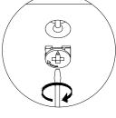
STEP 1 - USE A CROSS SLOT SCREWDRIVER TO TIGHTEN THE CAM BOLT INTO THE HOLE.
